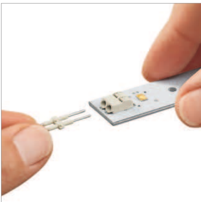
Inserting board-to-board link into terminal block.
