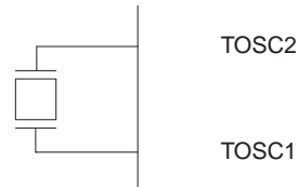
Figure 7-3. Crystal Oscillator Connections
