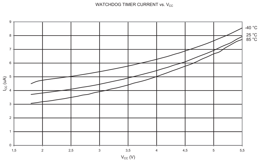
Figure 17-50. Watchdog Timer Current vs. V_{CC}
