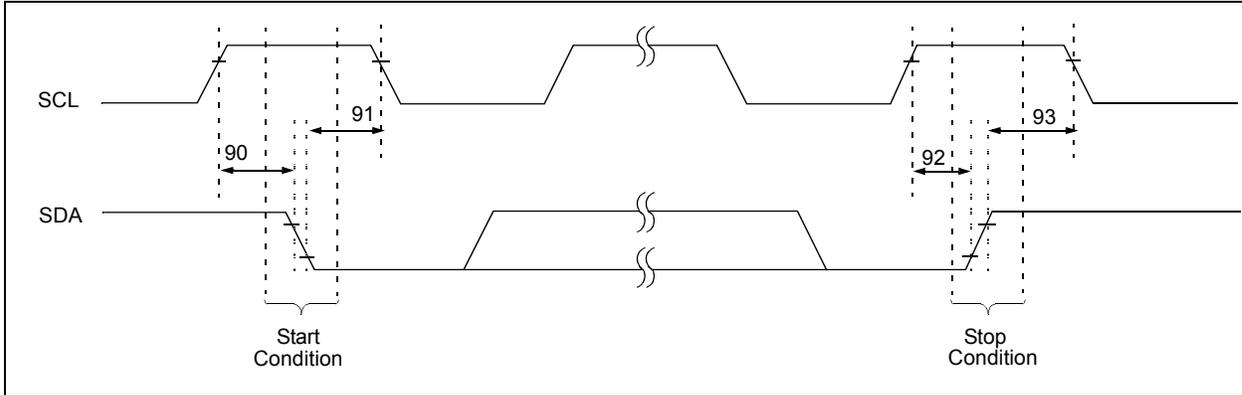
**TABLE 28-18: I<sup>2</sup>C™ BUS START/STOP BITS REQUIREMENTS (SLAVE MODE)**
