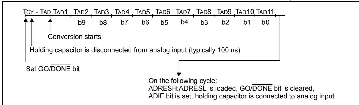
**FIGURE 20-4: A/D CONVERSION TAD CYCLES ( $\text{ACQT}<2:0> = 010, \text{TACQ} = 4 \text{TAD}$ )**
