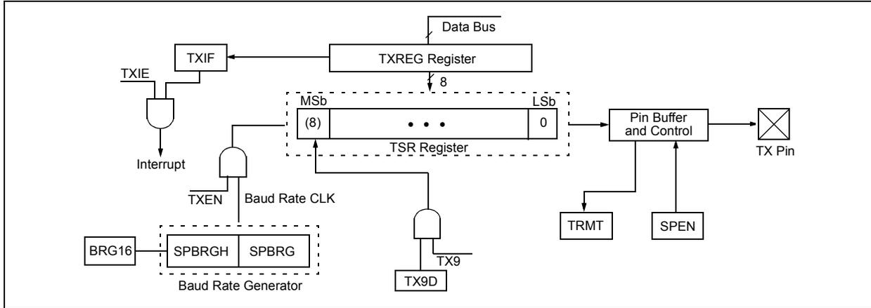
**FIGURE 19-4: ASYNCHRONOUS TRANSMISSION**
