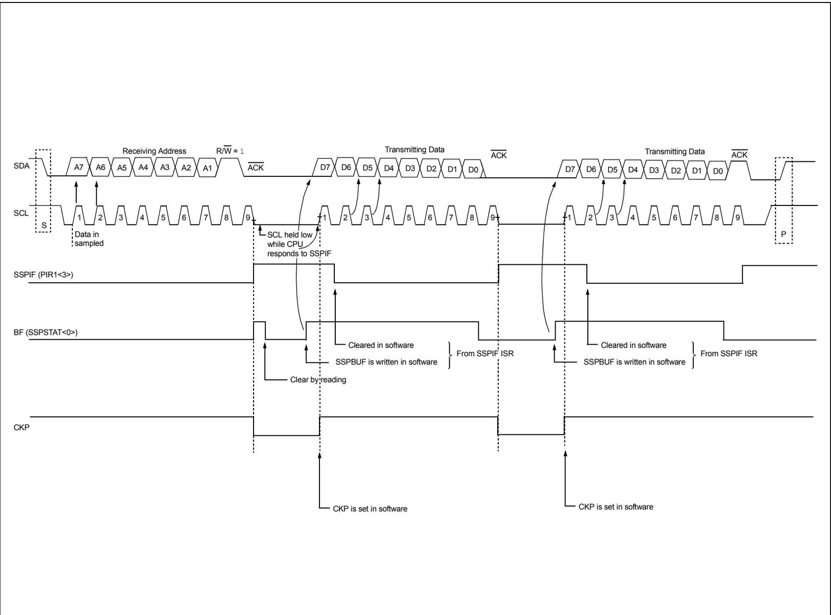
FIGURE 18-10: I<sup>2</sup>C™ SLAVE MODE TIMING WITH SEN = 0 (RECEPTION, 10-BIT ADDRESS)
