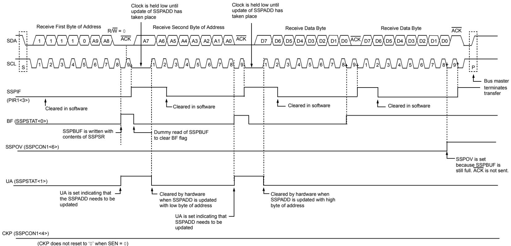
FIGURE 18-11: I<sup>2</sup>C™ SLAVE MODE TIMING (TRANSMISSION, 10-BIT ADDRESS)
