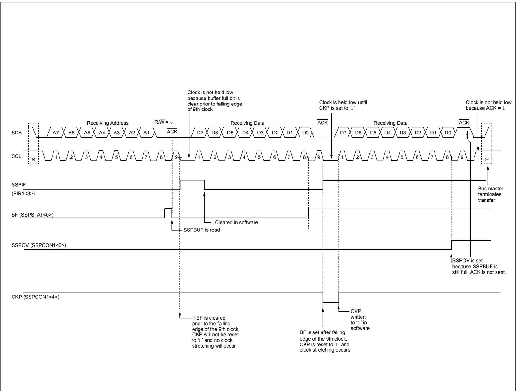
FIGURE 18-14: I<sup>2</sup>C™ SLAVE MODE TIMING SEN = 1 (RECEPTION, 10-BIT ADDRESS)
