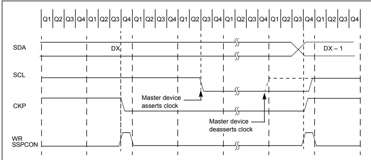
FIGURE 18-13: I<sup>2</sup>C™ SLAVE MODE TIMING WITH SEN = 1 (RECEPTION, 7-BIT ADDRESS)
