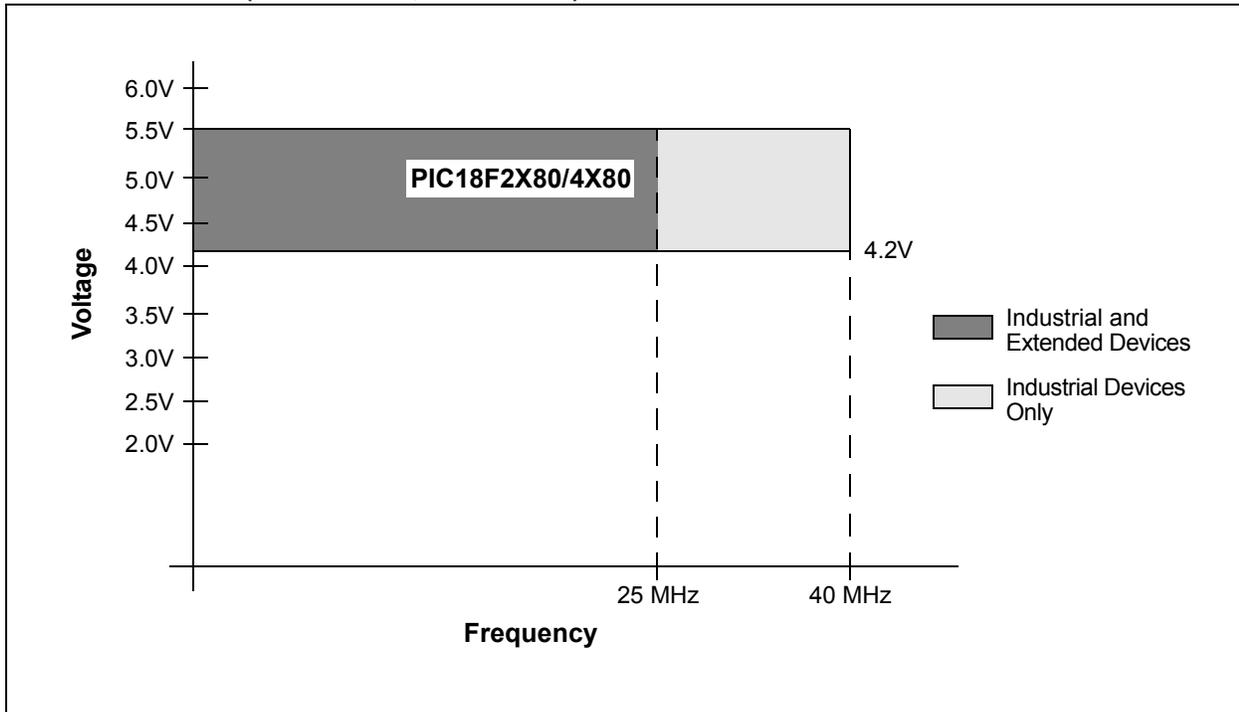
**FIGURE 28-2: PIC18LF2480/2580/4480/4580 VOLTAGE-FREQUENCY GRAPH (INDUSTRIAL)**
