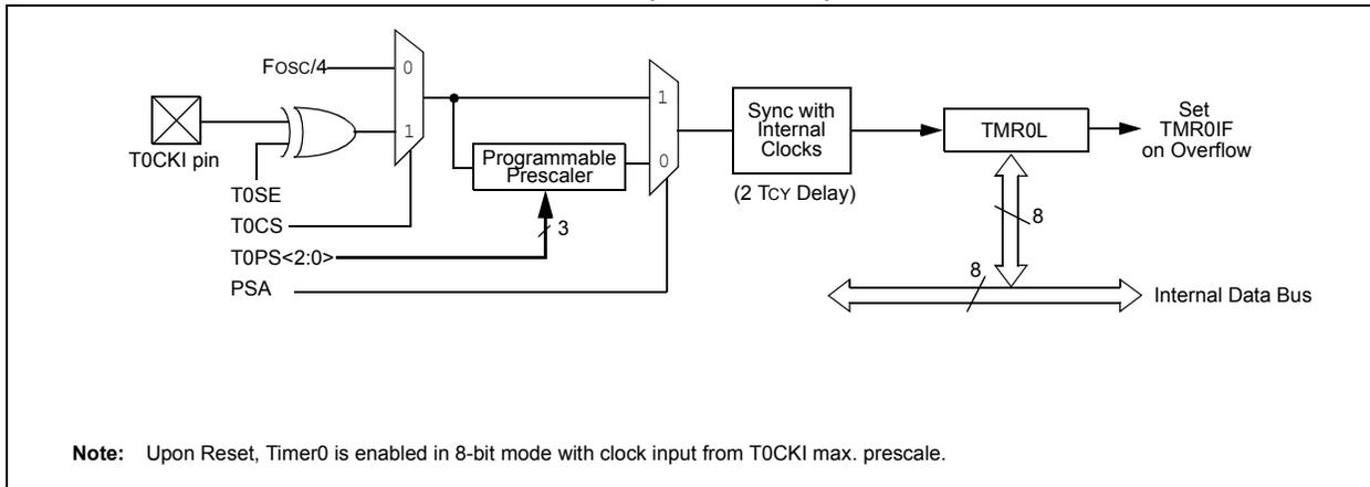
**FIGURE 12-2: TIMER0 BLOCK DIAGRAM (16-BIT MODE)**
