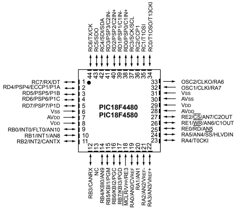
**Note 1:** For the QFN package, it is recommended that the bottom pad be connected to Vss.
