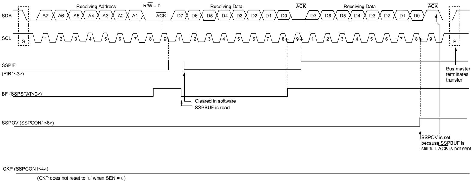
FIGURE 18-9: I<sup>2</sup>C™ SLAVE MODE TIMING (TRANSMISSION, 7-BIT ADDRESS)
