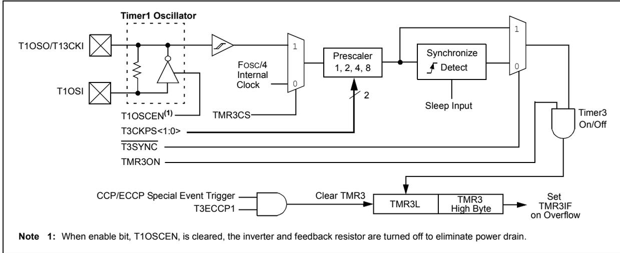
**FIGURE 15-2: TIMER3 BLOCK DIAGRAM (16-BIT READ/WRITE MODE)**
