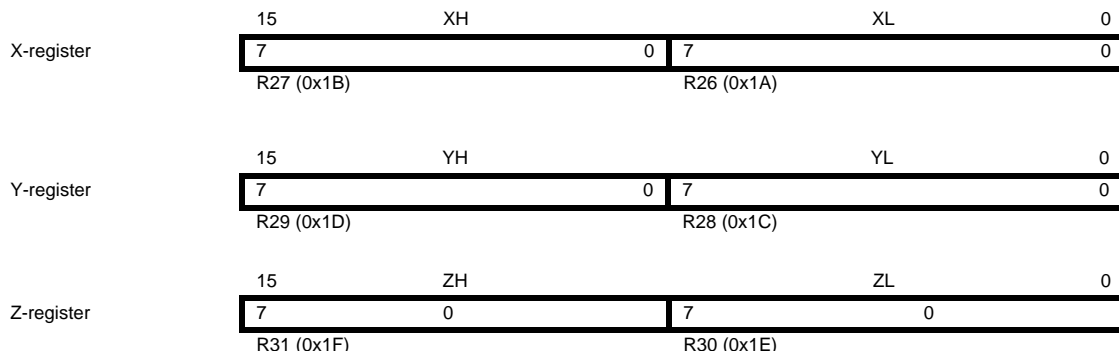
Figure 6-3. The X-, Y-, and Z-registers
