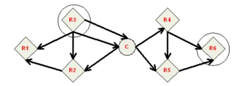
When the destination node receives a route request, it compares the 'path cost' field against previously received route request commands. If the path cost stored in the route request is better than any previously received, the destination node transmits a route reply packet to the node that originated the route request. Intermediate nodes receive and forward the route reply packet to the source node (the node that originated route request).
