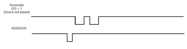
The following image illustrates the behavior pressing the button once on a remote device, causing a broadcast node identification transmission to be sent. All devices that receive this transmission blink their associate pin rapidly for one second if the associate LED functionality is enabled (D5 = 1).
