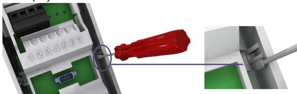
Figure 3 – Removing the Main Unit
