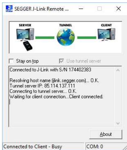
J-Link Remote Server: Connected to SEGGER tunnel server
