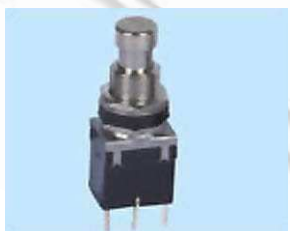
PS24102P ON-ON PS24112P ON-(ON) 4 A 125 VAC; 2 A 250 VAC SPDT 3P (L=14.2, 11.8, 9.8)
