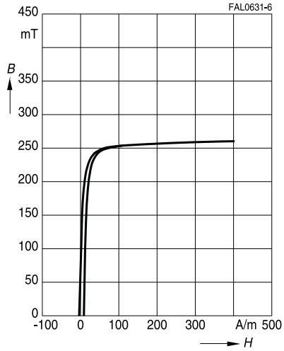
Dynamic magnetization curves (typical values) ( f = 10 \text{ kHz} , T = 100 \text{ °C} )
