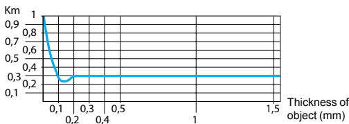
Typical curve for a copper object used with a \varnothing 18 mm cylindrical sensor
