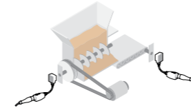
Detection of underspeed, shaft overload
