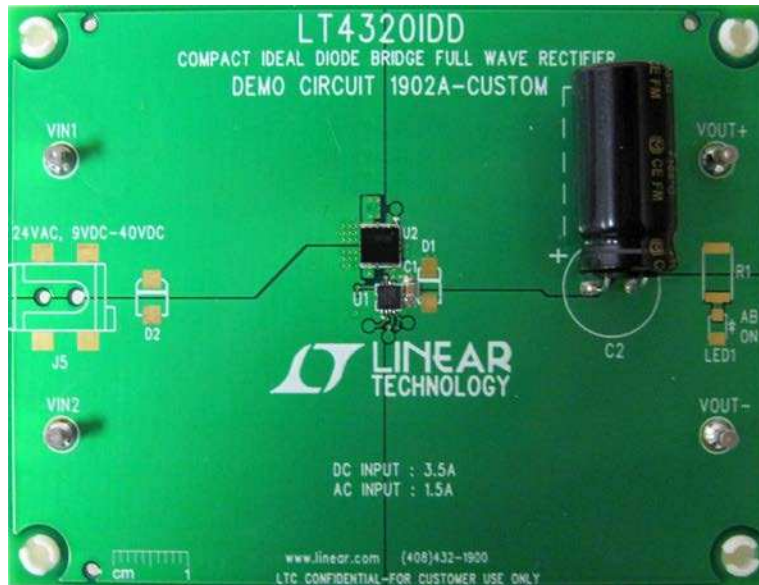
Figure 4. Demonstration Circuit 1902A Used in Figure 3 Thermograph
