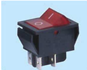
RSI2011B ON-OFF RS2011B ON-OFF DPST 4P
