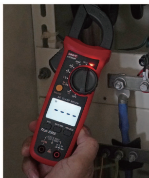
NCV multi-segment display and audio/visual alarm
