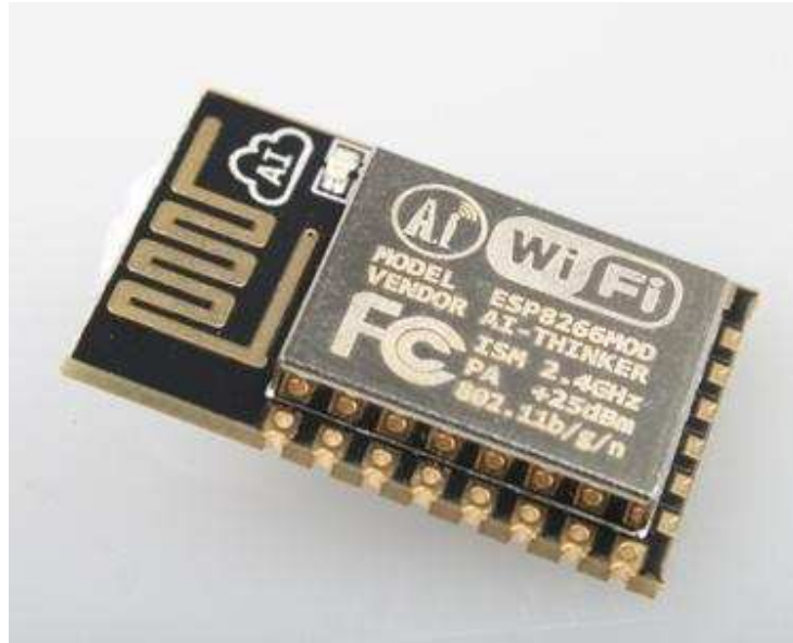
Figure 3 [Module Pin Counts, 22 pin, 16 mm *24 mm *3 mm]
