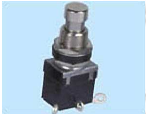
PS24102 ON-ON PS24112 ON-(ON) 4 A 125 VAC; 2 A 250 VAC SPDT 3P (L=14.2, 11.8, 9.8)
