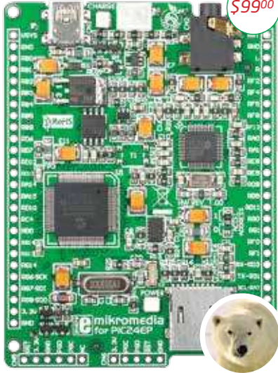
mikromedia for PIC24EP (features PIC24EP512GU810)
