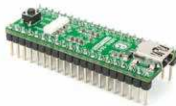
MIKROE-1368 MINI-M4 for Stellaris contains LX4F230H5QR (ARM ® Cortex ™ -M4)
