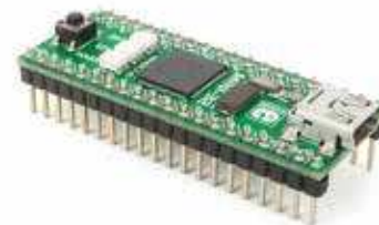
MIKROE-763 MINI-32 contains PIC32MX534F064H
