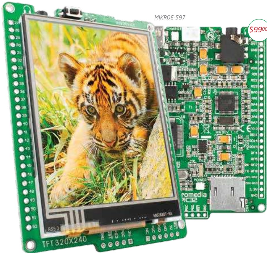
mikromedia for PIC32 (features PIC32MX460F512L)
